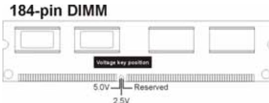
Install the 184-pin DDR SDRAM modules in any combination as follows:
