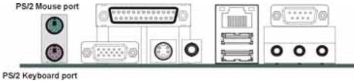
Connect a PS/2 keyboard to the purple 6-pin mini DIN connector. If you want to connect a standard AT size (large DIN) connector, you must use an adapter.
