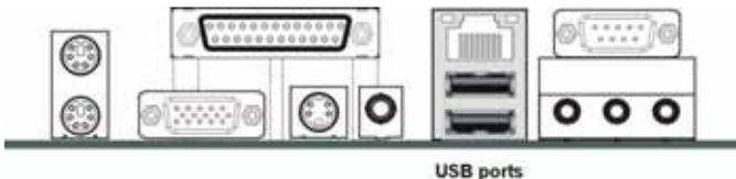
The USB ports provide a hardware interface for low-speed peripherals such as the keyboard, mouse, joystick, scanner, printer and telephony devices, and also support MPEG-1 and MPEG-2 digital video. The USB ports have a maximum bandwidth of 480 Mbits/sec (equivalent to 60 Mbytes/sec), and up to 127 devices can be attached. Fast devices can use the full bandwidth, while lower-speed ones can transfer data using a 60 Mbytes/sec sub-channel.
