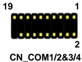
**Connector:** CN\_COM1/2**Type:** 20-pin (10x2 pitch=1.27x2.54mm) header
