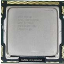
Intel® i3/i5/i7® processor Package type: 1155 pin FCLGA FSB:1066/1333MHz
