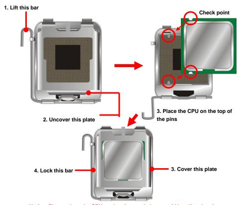
Notice: Please place the CPU on the pins tenderly to avoid bending the pins
