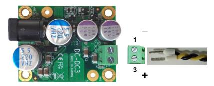
DC\_OUT: Terminal Block 2-pin power connector
