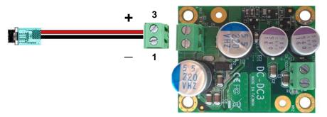
DC\_IN: Terminal Block 2-pin power connector
