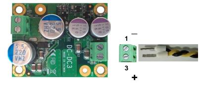
**DC\_OUT**: Terminal Block 2-pin power connector
