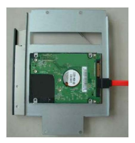
16. Turn the CD-ROM driver screws and SATA cable connects well and turn the screws.
