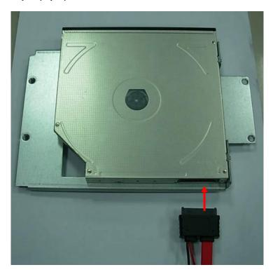
11. After install HD driver, Turn the CD-ROM holder and front panel screw well. Refer picture A and B.
