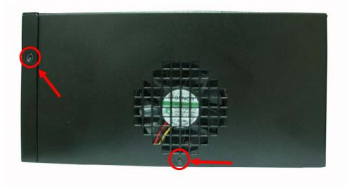
2. Push the Chassis shield towards the back then open it.
