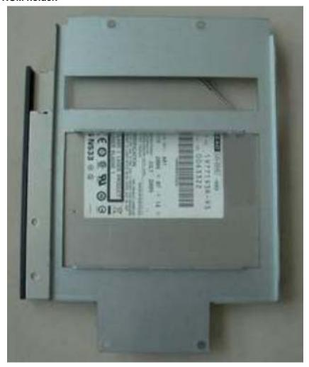
14. Put on HD driver into HD holder then turn the HD drive screws to tighten. Refer picture A , B and C.
