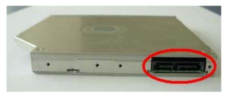
10. Check the CD-ROM driver and SATA cable connects well, then connect the ATX output (4-pin).
