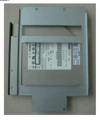
14. Put on HD driver into HD holder then turn the HD drive screws to tighten. Refer picture A , B and C.
