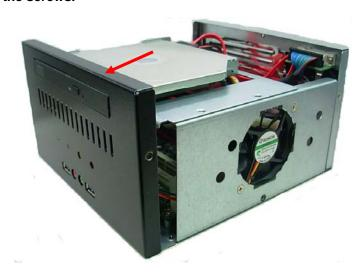
17. Turn the chassis shield screws to tighten well.
