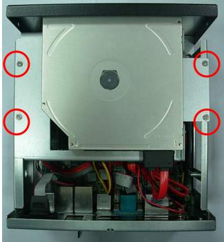
18. Turn the chassis shield screws to tighten well.
