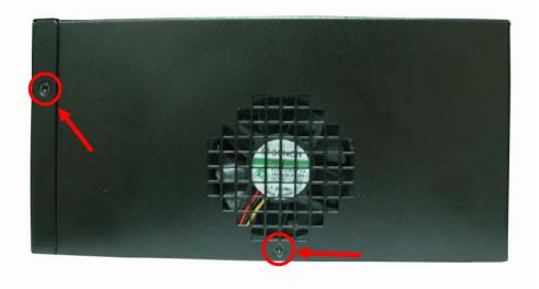
3. Push the Chassis shield towards the back then open it.
