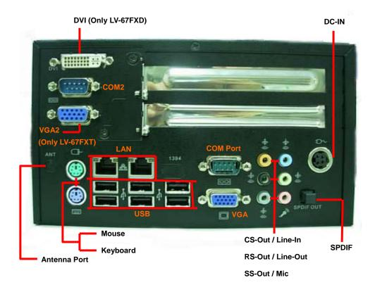
Power input: DSPD-080-12A 80W 12V AC-DC Adapter Input.
