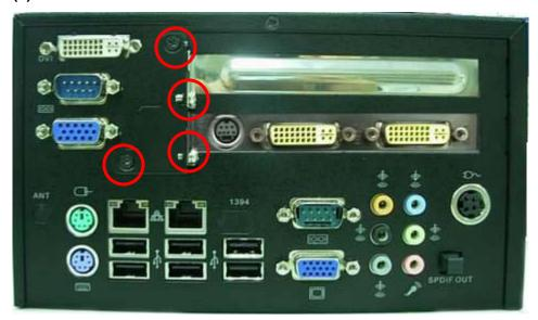
10. After install HD driver, Turn the CD-ROM holder and front panel screw well refer picture.
