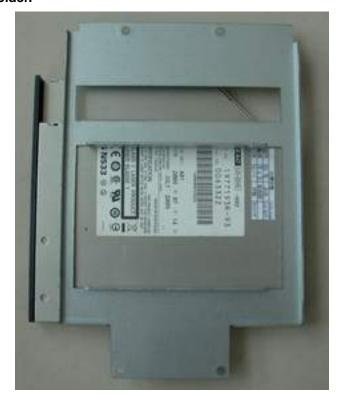
Put on HD driver into HD holder then turn the HD drive screws to tighten. Refer picture  ${\bf A}$ ,  ${\bf B}$  and  ${\bf C}$ .
