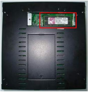
8. Press down the memory module then check dimm holder hook well.
