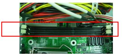
5. Press down the memory module then check dimm holder hook well.
