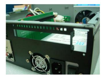
7. Put into the PCI-E Card. And Check the connects into the riser card well then turns shield screw.
