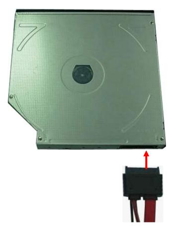
13. Insert CD-ROM into the chassis from front panel.
