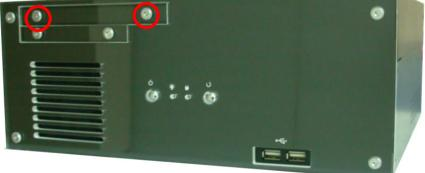
3. Open the CPU cover and refer the motherboard manual page.15 to install the CPU.
