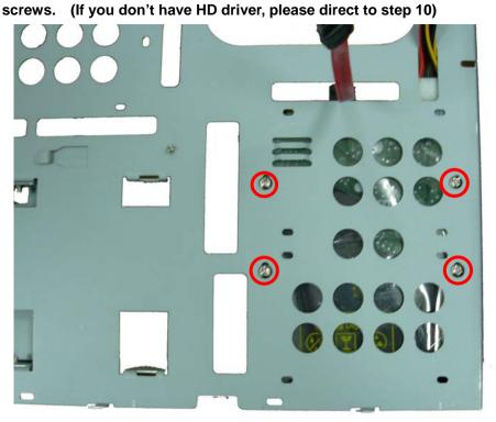
10. Before Install the CD-ROM. Turn the CD-ROM shield screws and take it off.
