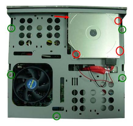
15. To tighten the chassis shield screws well.
