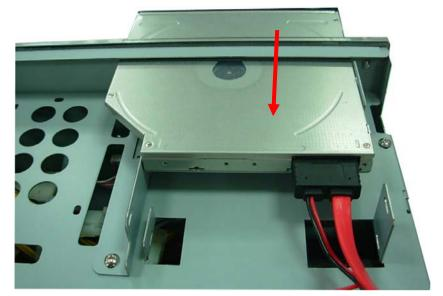
14. To tighten the CD-ROM and holder screws.
