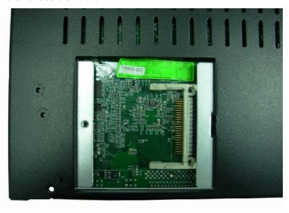
3. Follow the Idiot-proof design then insert the CF card, Check connected well.
