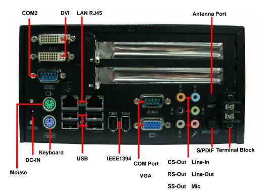
**Power input**: DSPD-080-12 80W 12V AC-DC Adapter or Terminal Block 12V DC Input.
