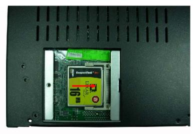
4. Close CF chassis shield and turn screw to tighten.
