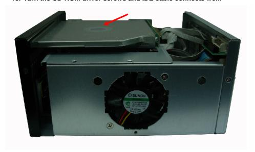
19. Turn the chassis shield screws to tighten well.
