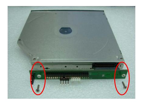
12. Turn the CD-ROM driver screws and IDE cable connects well.
