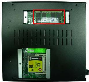
8. Press down the memory module then check dimm holder hook well.
