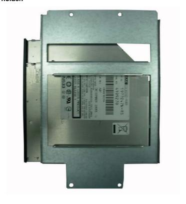
16. Put on HD driver into HD holder then turn the HD drive screws to tighten.(If you don't have HD drive please direct to step.18)
