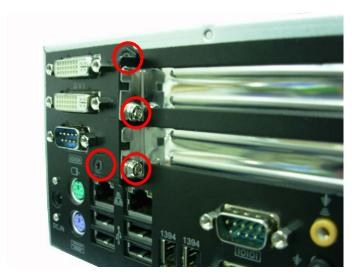
(B). You can install Riser-Card PCI-2P1 PCI card.
