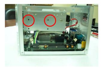
9. Please screw up the HDD bay and connect SYS FAN cable on the CN\_SYSFAN .
