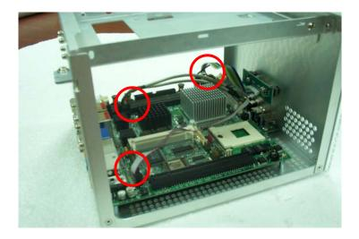
8. Before install HDD drive bay on the chassis , please screw up HDD drive .
