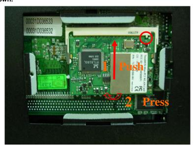
4. To close mini-PCI chassis shield and tighten a screw.
