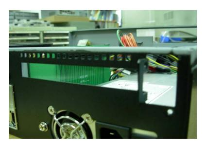
9. Put into the PCI-E Card. And Check the connects into the riser card well then turns shield screw.
