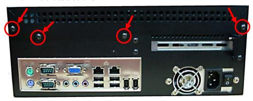
2. Push the Chassis shield towards the back then open it .
