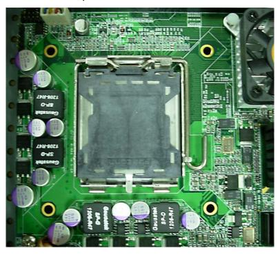
6. Open the Dimm holder then check the pin number to match the socket side well before installing memory module.
