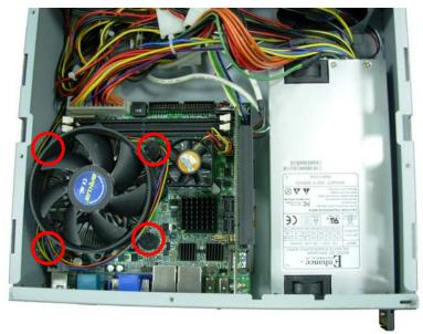
5. Open the CPU cover and refer the motherboard manual page.16 to install the CPU.
