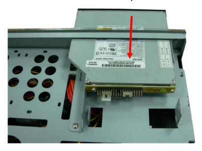
17. To tighten the CD-ROM and holder screws.
