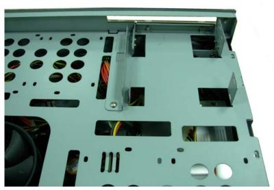
16. Insert CD-ROM into the chassis from front panel.
