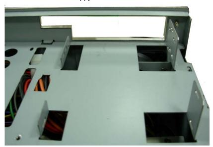
14. Turn the floppy Screws then refer motherboard manual page "21" to connect the floppy cable correctly.
