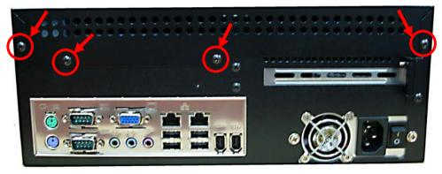
2. Push the Chassis shield towards the back then open it .
