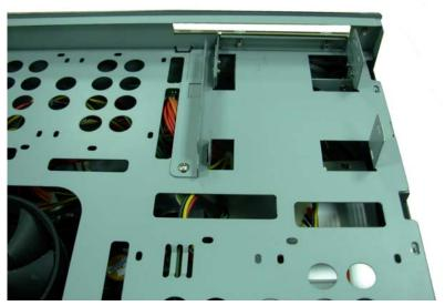
16. Insert CD-ROM into the chassis from front panel.
