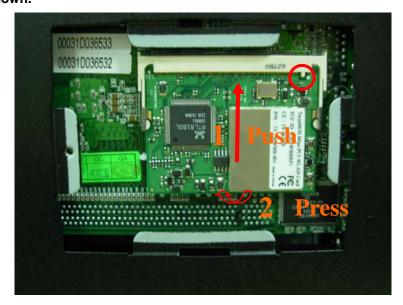
4. To close mini-PCI chassis shield and tighten a screw.
