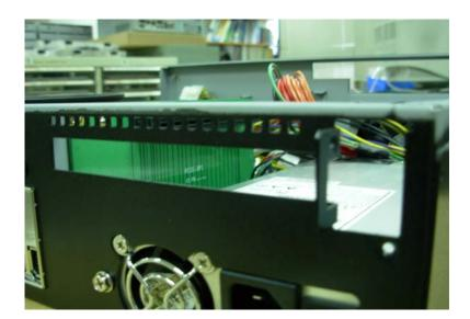
9. Put into the PCI-E Card. And Check the connects into the riser card well then turns shield screw.
