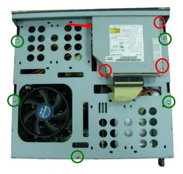
18. To tighten the chassis shield screws well.
