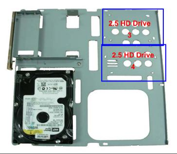
11. Put into HD driver and connect the cable well then turn the HD driver screws. (If you don't have HD driver, please direct to step 12.)
