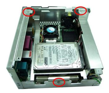
5. Check the fan below the HDD drive bay, and connect the cable on CN\_SPWR.
