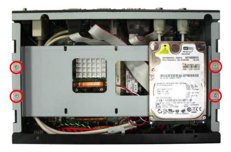
8. Push the Chassis shield towards the back then open it.
