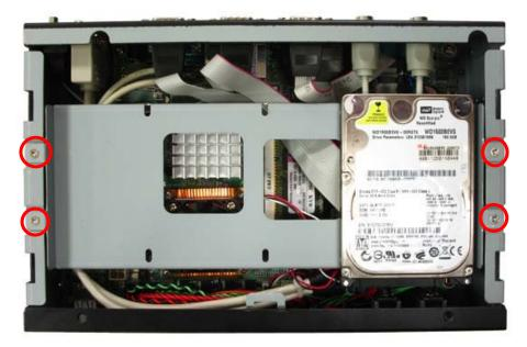
Turn the CPU cooler screws and then refer the motherboard manual page.17 to install the CPU.(After installing CPU, please turn the CPU FAN screws to tighten.)
