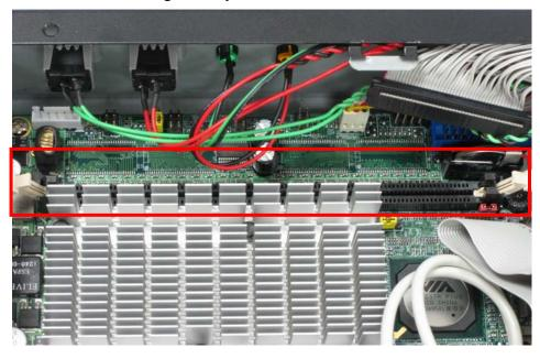
5. Press down the memory module then check DIMM holder hook well.
