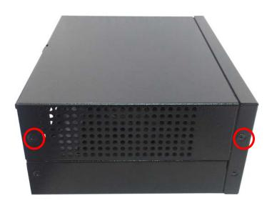
2. Push the Chassis shield towards the back then open it.
