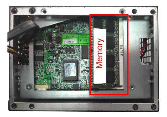
(B) Press down the memory module then check dimm holder hook well.
