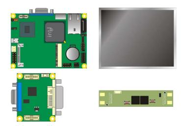
Please check the datasheet of the panel to see the voltage of the panel, and set the jumper JVLCD(LP-170) to +5V or +3.3V.
